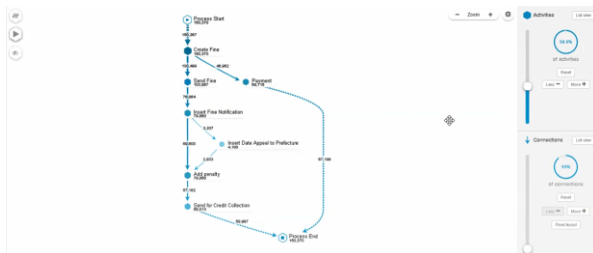
Figure 1. DFG in the “Process Explorer” in Celonis. The sliders on the right allow users to change the level of detail for the graph. Annotations can be changed by selecting the top left icon. Here also custom metrics can be defined.
